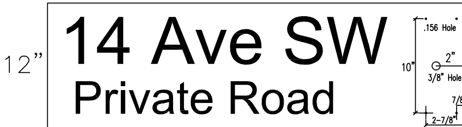
D3-3PVT 12x36 Copy - Line 1 - 6 Inch Highway Gothic Series B Line 2 - 3 Inch Highway Gothic Series B Silver Legend on a Green Background
