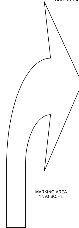
TYPE 2R (RIGHT) TRAFFIC ARROW MIRROR IMAGE OF TYPE 2L TRAFFIC ARROW
