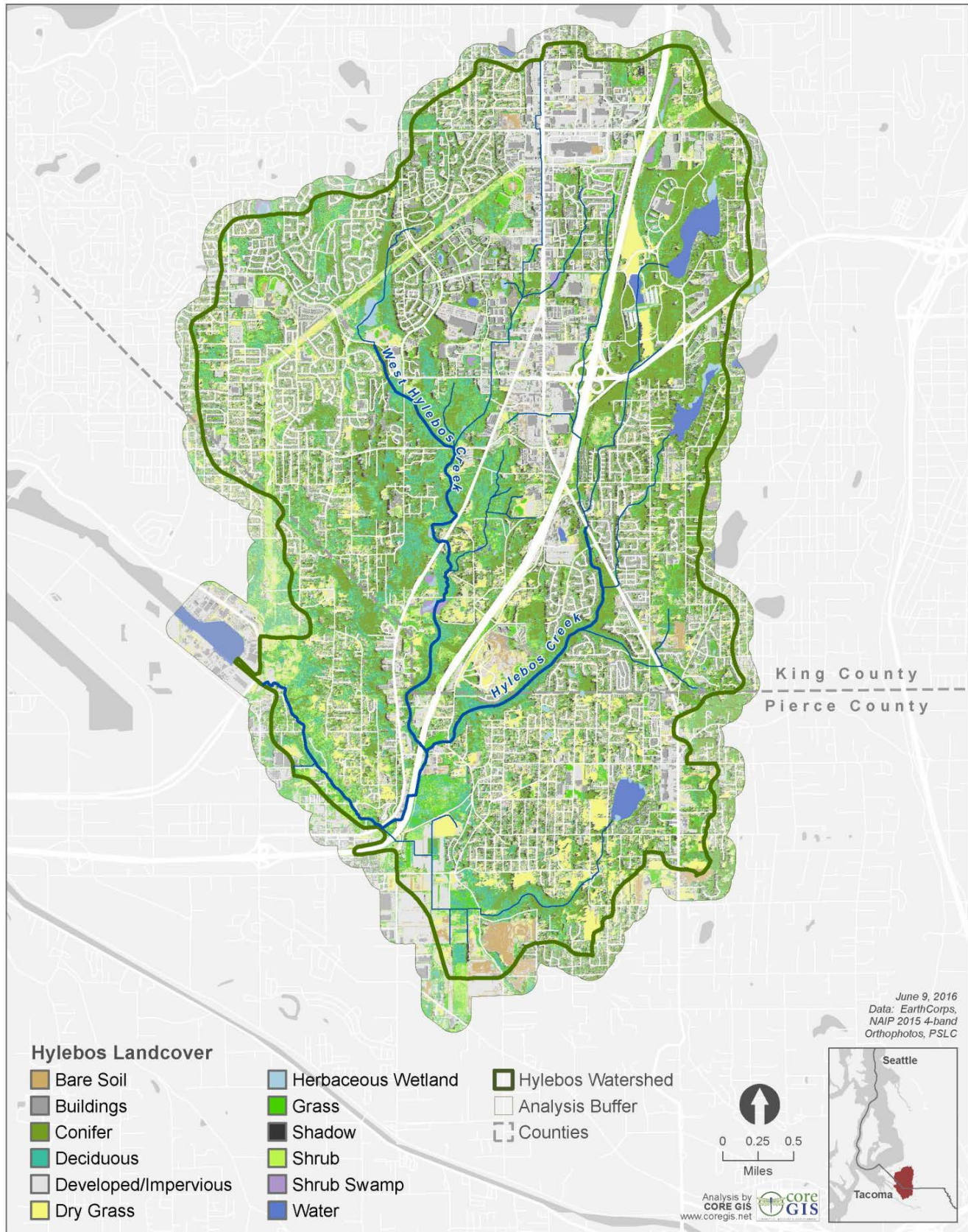
Figure 27: Land cover types in the Hylebos watershed derived from remote GIS analysis based on 2015 orthophotography.
